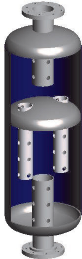
Figure 1.0 Typical Burgess-Manning reactive type silencer
