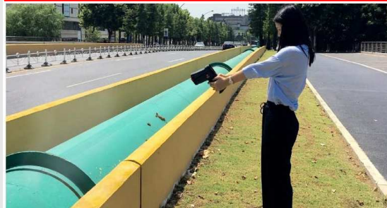
Natural Gas Pipeline Gas Leak Inspection
