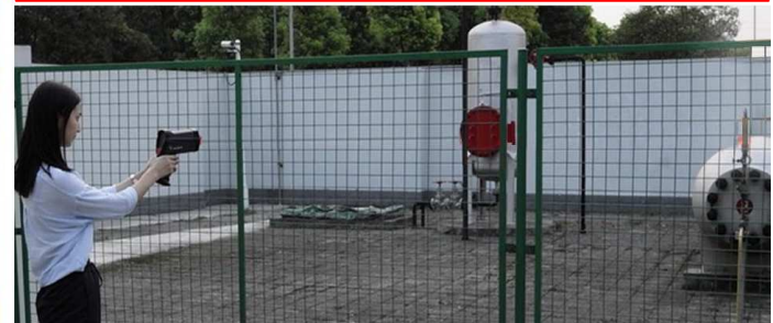
Gas Container Methane Leak Inspection
