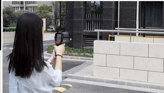
Residential Building Natural Gas Leak Inspection
