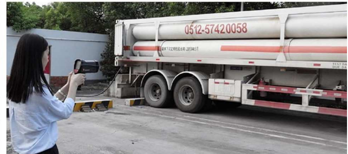
Gas Container Methane Leak Inspection
