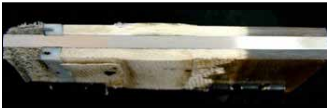
Steam attack on GRE isolation gasket
