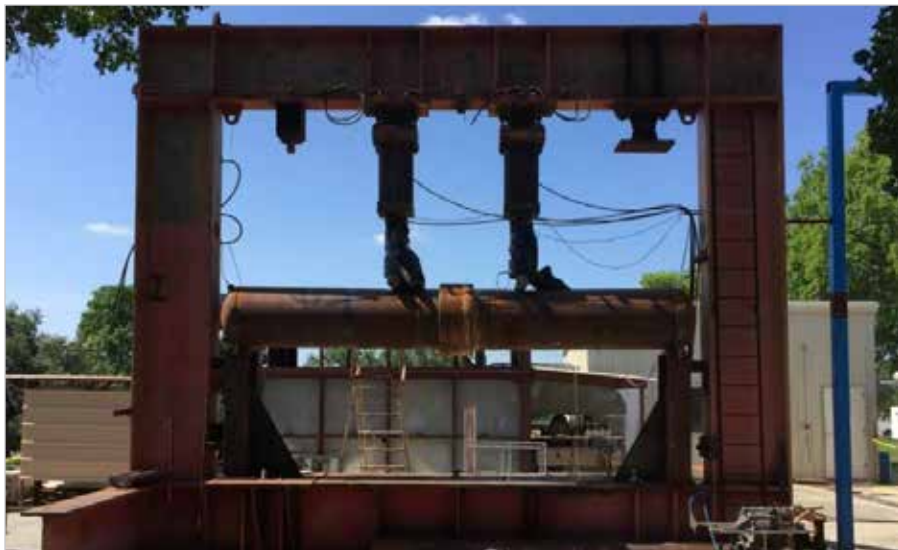
HYRDO-BENDING TEST - SOUTHWEST RESEARCH INSTITUTE
