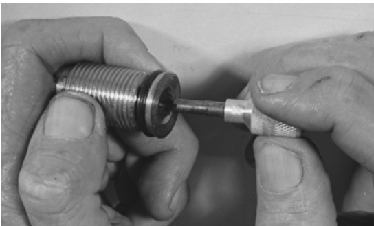
Figure 5. Check Tightness of Valve Core
